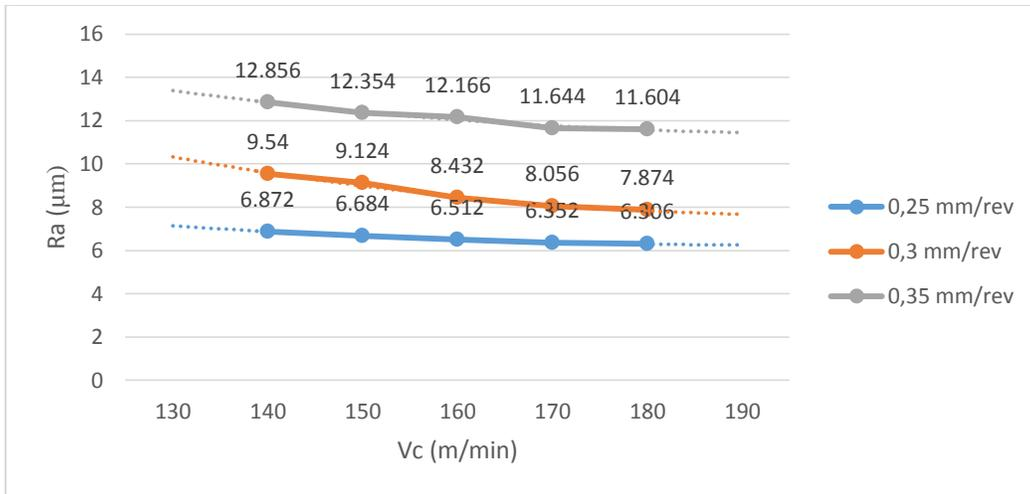
Figure 7. Graphic Cutting Speed Vs Surface Roughness
