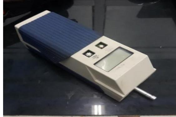
Figure 3. Surface Tester Mitutoyo 211
