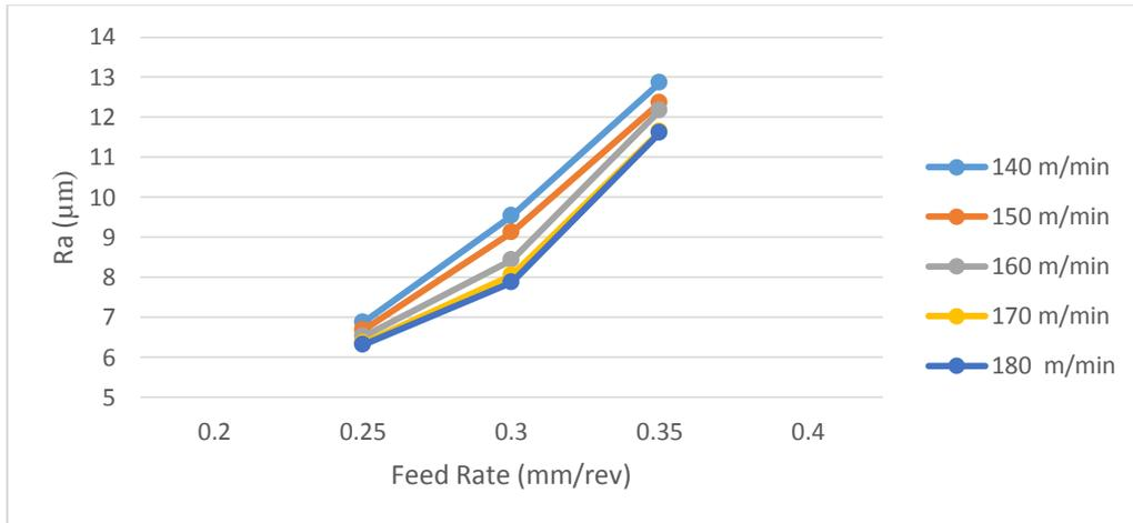
Figure 6. Graphic Feed Rate vs Surface Roughness
