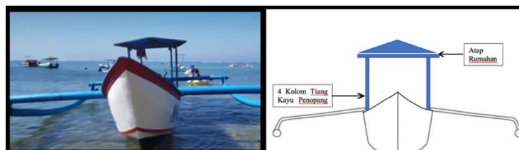
Figure 8. A Triangular Roof With Four Pillars
