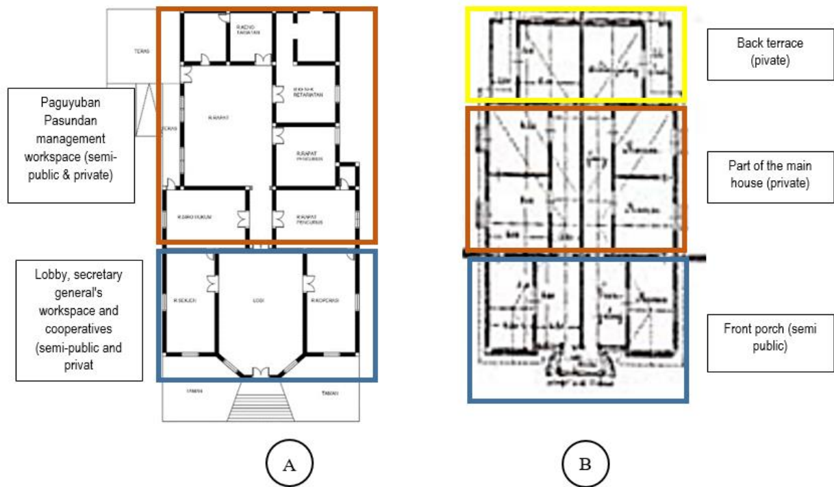
Figure 7. Comparison of the condition of the Paguyuban Pasundan building concerning the colonial residence plan for an officer with the rank of Lieutenant
