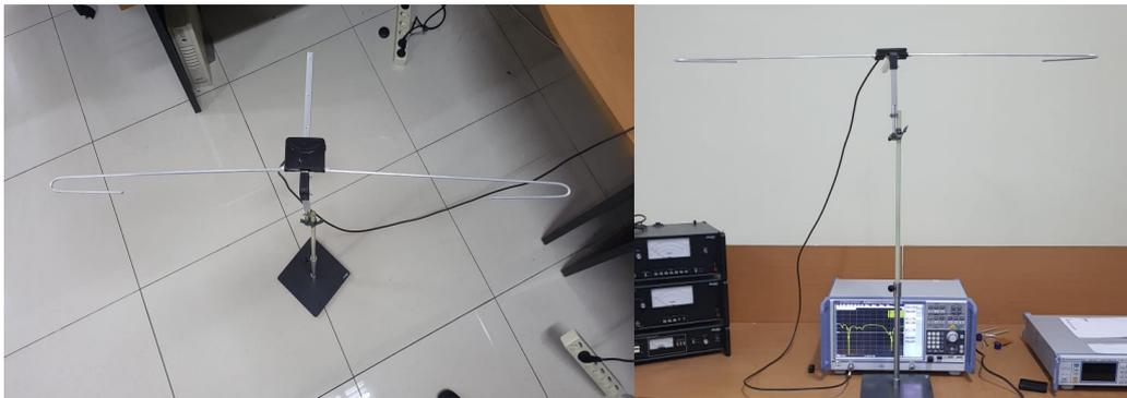
Gambar 10. Fabrikasi antenna *dual band dipole folded end*
