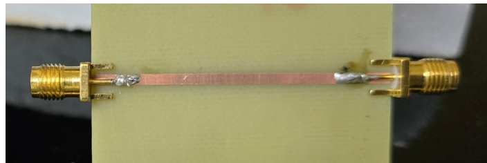
Figure 3. Fabricated microstrip line in FR4 substrate with two SMA connectors.
