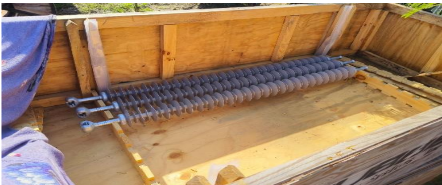
Gambar 2. 5 Isolator Polymer SUTT 70 kV GI Namlea – GI Namrole
