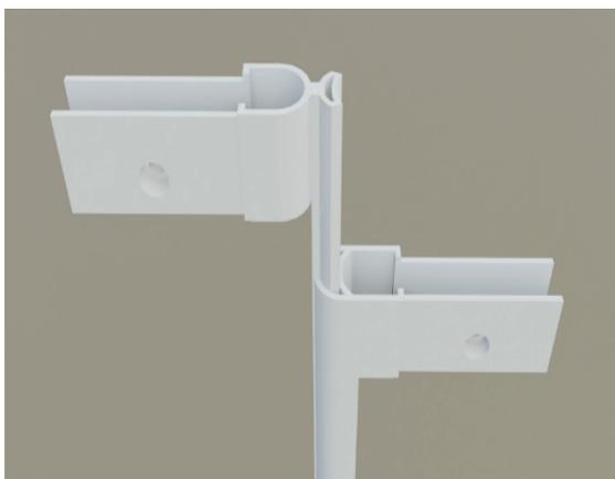
Gambar 13 Render 3D Engsel Lift
