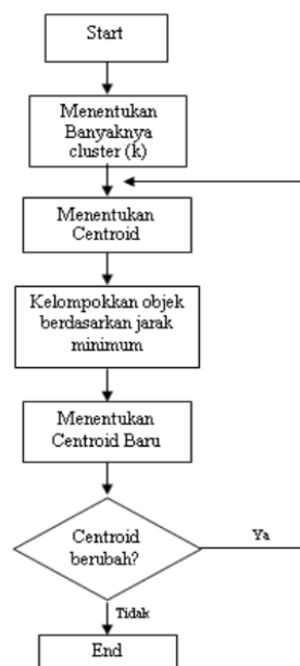
Gambar 2. Tahap Algoritma Clustering K-Means [14]
