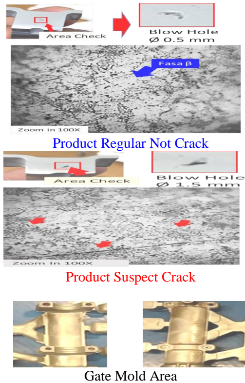
Fig. 4. Comparative analysis of cracks and no cracking phenomenon
