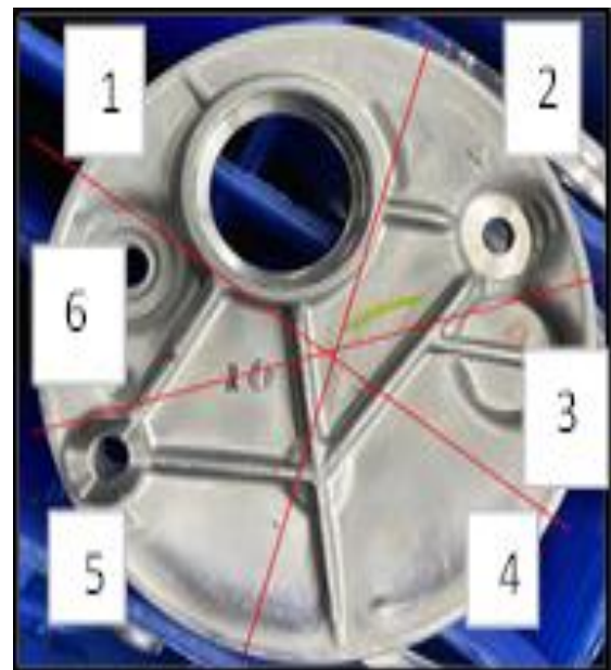
Fig. 1. Defect position for point 1 to 6
