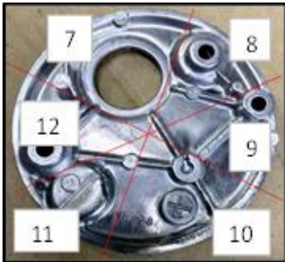
Fig. 2. Defect position for point 7 to 12
