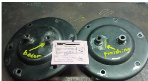
Figure 1. Types of leaking defects and untidy finishing
