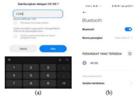
Fig. 3. (a) Identification of the Bluetooth Sensor on the Smartphone, (b) HC-05 Bluetooth Sensor Connects Successfully with the Smartphone
