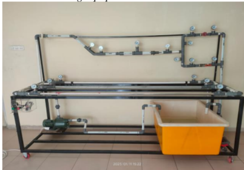
Fig. 25. Head loss testing equipment
