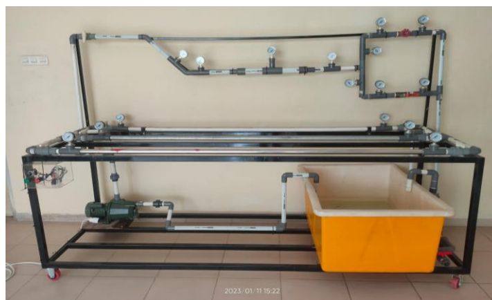
Figure 26. Head loss testing equipment
