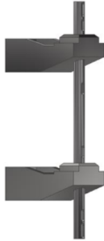
Fig 6. 3D Assembly Hub Bearing Sprocket and Shaft with Autodesk Inventor Pro 2019 Software
