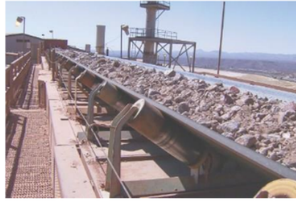
Figure 1. Illustration conveyor belt. length 223 m, belt width 750 mm.
