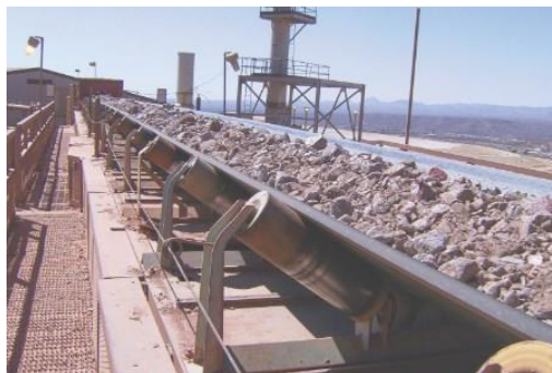
Figure 1. The conveyor belt system analyzed in this study, with a total length of 223 meters and a belt width of 750 mm
