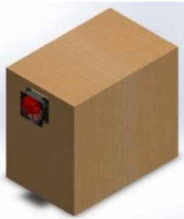
Figure 4. Sound acoustic compressor enclosure design
