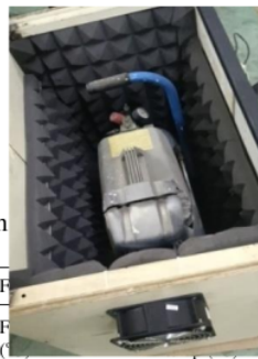
Figure 4. Sound acoustic compressor enclosure design
