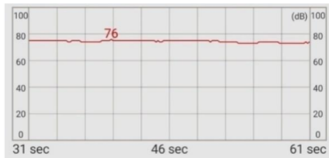
Figure 8. Sound level compressor measurement after using enclosure
