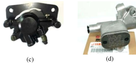
Figure 2. Brake component a) Diskbrake, b) Hose Brake c) Caliper dan d) Brake Master
