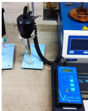
Figure 9. Setup for kinematic viscosity analysis
