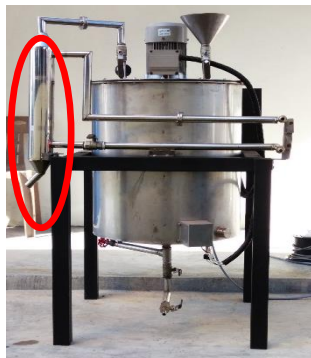
Figure 3. Location of Condensing Chamber
