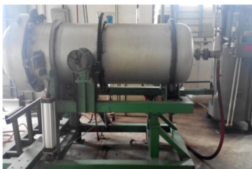
Fig. 2. The prototype of steam hyperbaric hydrothermal chamber
