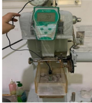
Figure 2 Denver flotation machine
