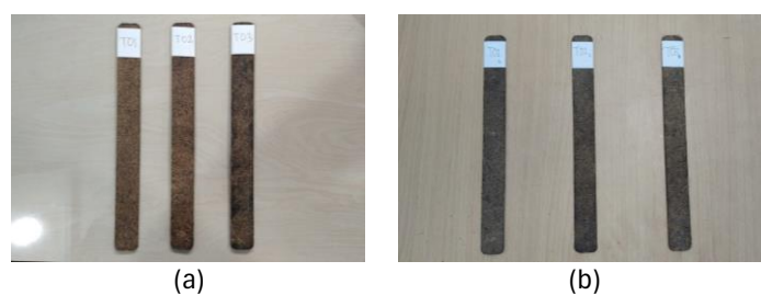
Figure 6. (a) Tensile test specimen, (b) Hardness test specimen
