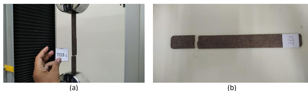
Figure 7. (a) Tensile test in progress, (b) Fractured specimen after testing
