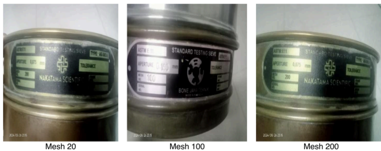
Figure 3. Filter Mesh Size
