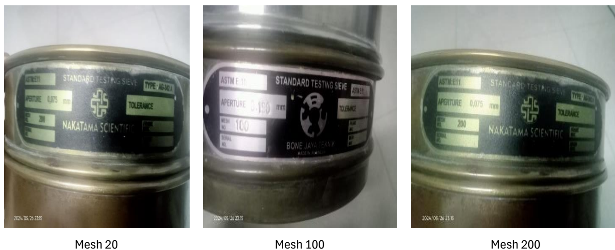
Figure 3. Mesh sieves used for particle size classification (Mesh 20, 100, and 200)
