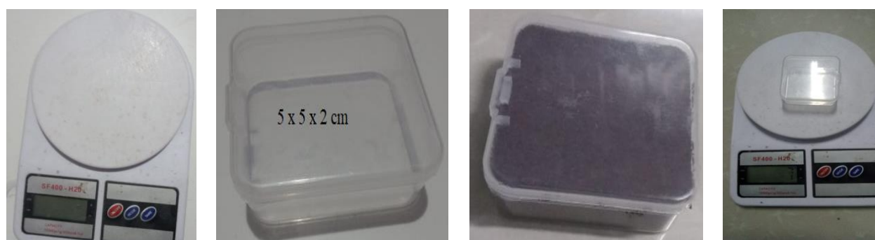
Figure 4. Measurement of container volume used for weighing coffee powder samples
