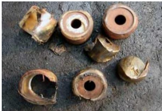
Figure 2. Damaged CVT roller weights in motorcycles [3].
