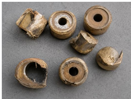
Figure 2. Illustrative example of damaged motorcycle CVT weight rollers.
