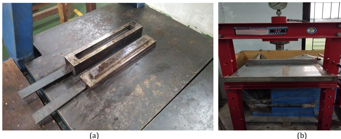
Figure 3. Equipment used for composite fabrication: (a) mold for preparing ASTM D3039 tensile-test specimens and (b) hydraulic hot-press machine.
