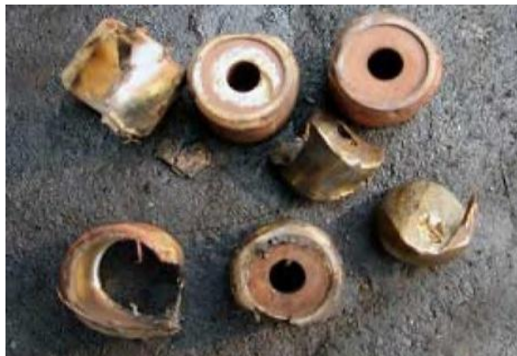
Figure 2. Damaged CVT roller weights in motorcycles [3].
