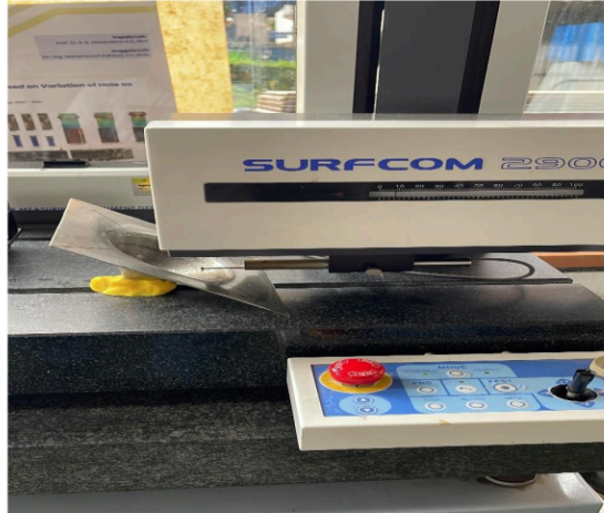
Figure 4: SURFCOM 2900 for surface roughness measurement
