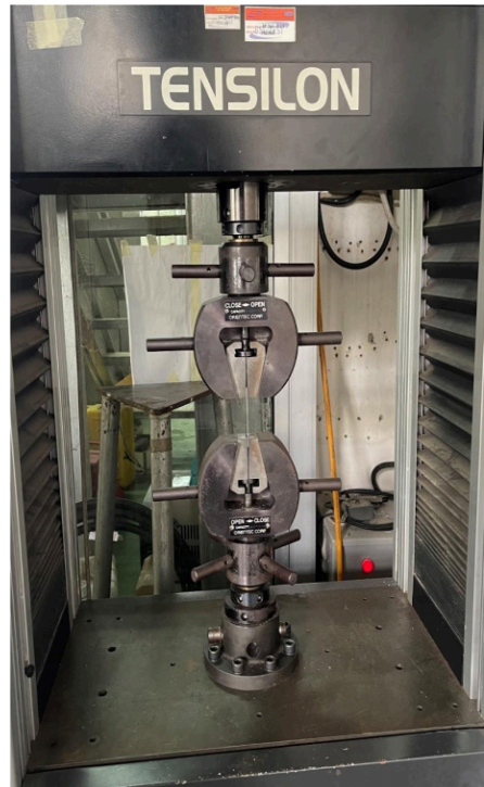
Figure 2: Tensilon RTF-2350 Universal Testing Machine
