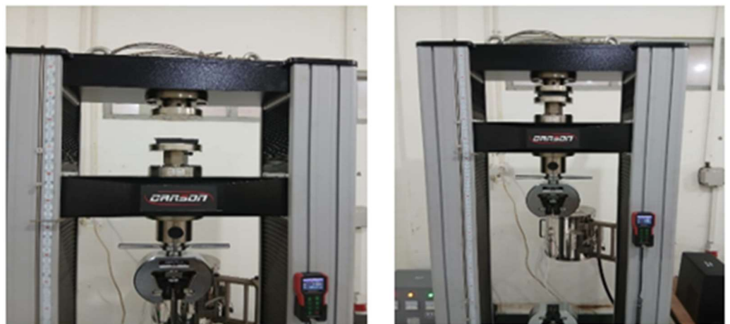
Figure 2. Composite Compression Test Using Universal Testing Machine Double Column Cap 20 Ton HK 2B FST
