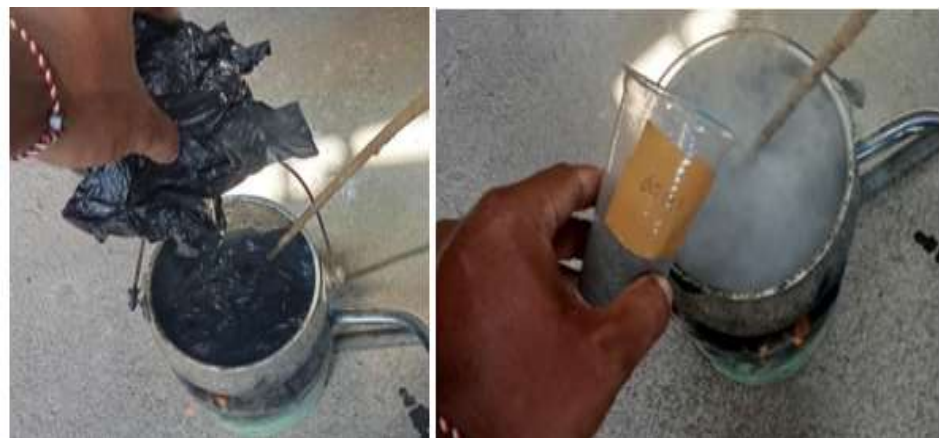
Figure 5. The process of melting PE waste and mixing rice husk ash
