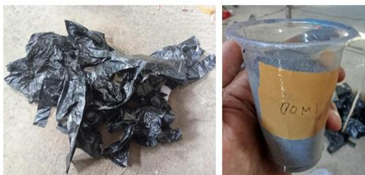
Figure 3. PE plastic waste and rice husk ash (RHA) used as raw materials for composite production
