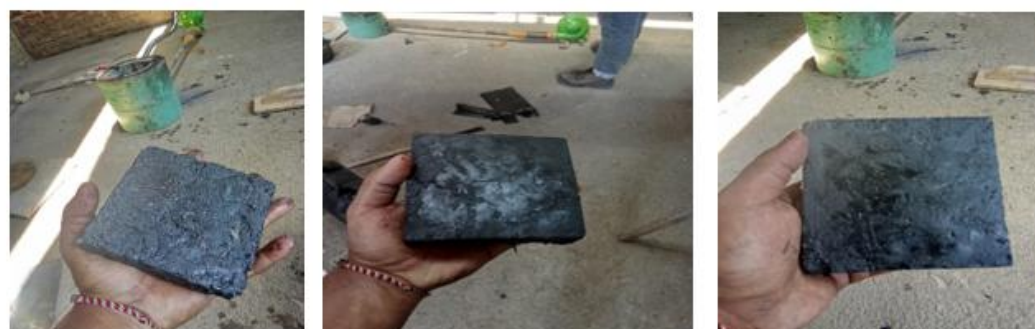
Figure 5. Fabricated PE-RHA composite specimens with composition ratios of 80:20, 70:30, and 60:40
