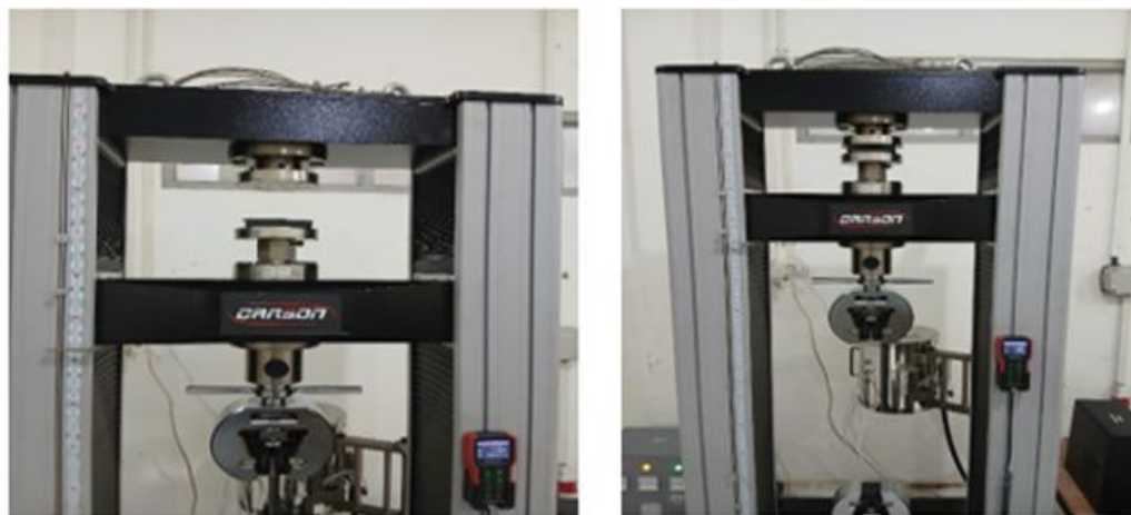
Figure 1. Compressive and tensile testing of composite specimens using a double-column universal testing machine with a 20-ton capacity
