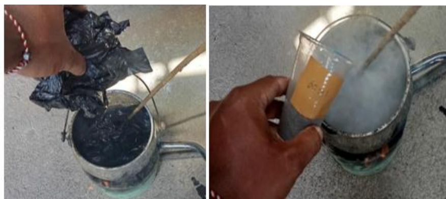
Figure 4. Melting of PE plastic waste and mixing with rice husk ash during the composite fabrication process
