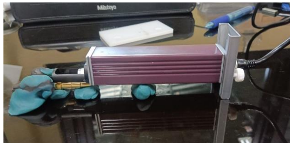
Figure 5. Surface roughness measurement procedure using the Mitutoyo SJ-310 tester.
