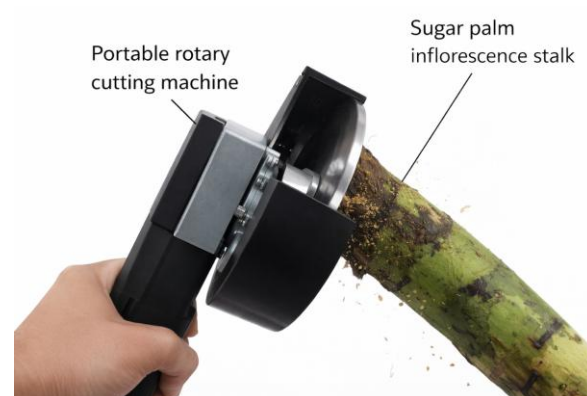
Figure 5. Experimental setup during machine-assisted trimming of sugar palm inflorescence stalk.
