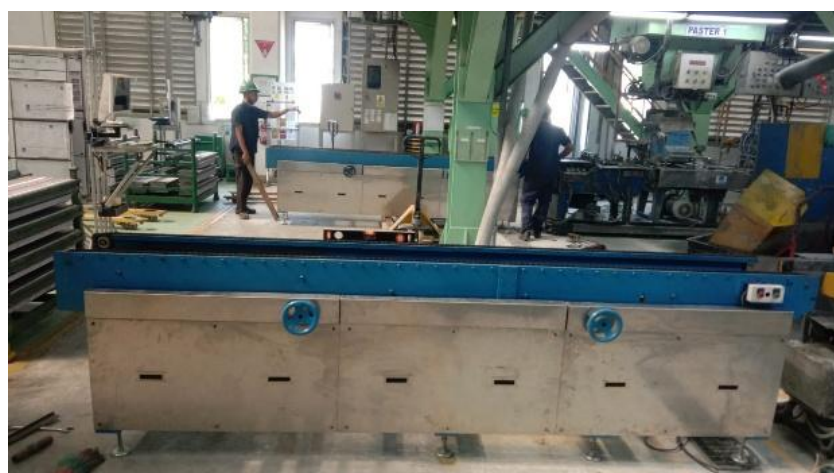
Figure 14. Chain conveyor grid feeder unit.
