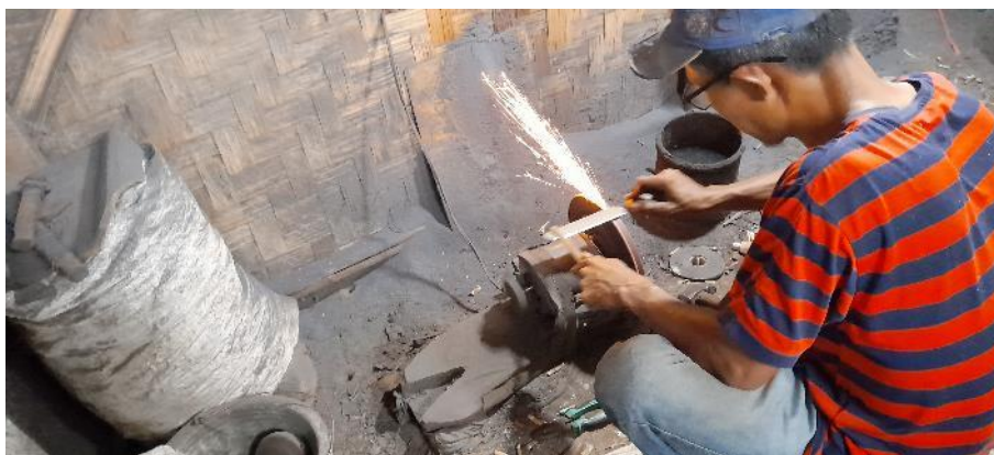
Figure 3. The craftsmen use simple tools to produce knives
