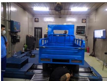
Gambar 2. Proses *dyno test*
