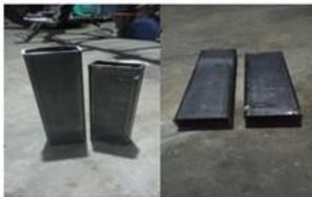
**Gambar 1.** Material SS400 Type Hollow Rectangle
