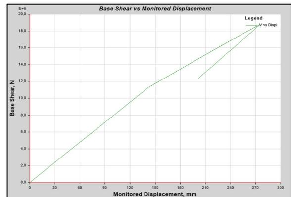
**Figure 10.** The capacity curve of 4-story soft soil SMRSF
