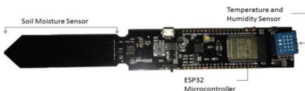
Figure 2. ESP32 for wireless sensor network nodal for agriculture application [35].
