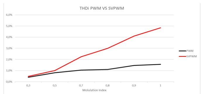
Figure 12. Graph THDi : of Pwm Vs Svpwm at frequency 50 Hz and modulation index 0.3 - 1.
