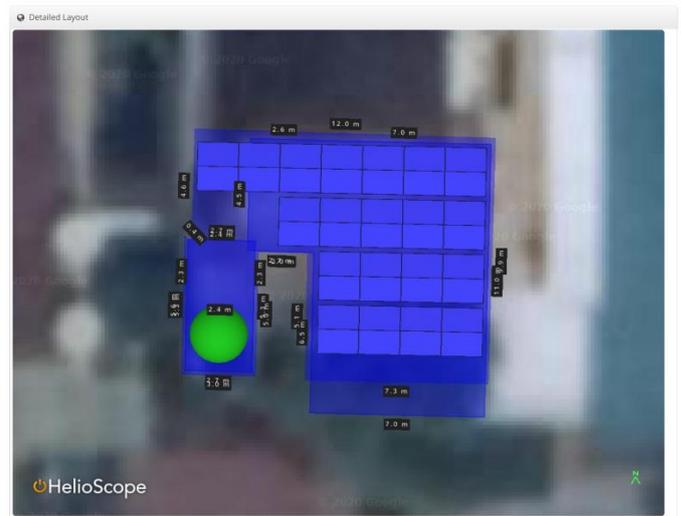
Gambar 4.4 Layout Design Perencanaan PV (Helioscope)
