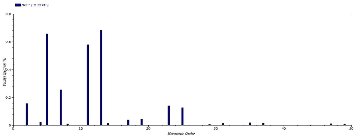
Figure 11. Harmonic Spectrum on Bus 2 After Mitigation
