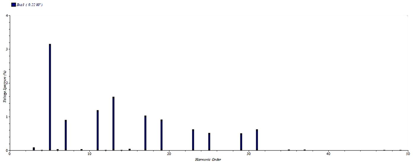
Figure 7. Harmonic Spectrum on Bus 1
