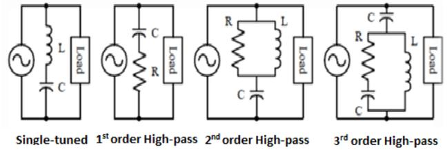
Figure 5. Types of Passive Filter
