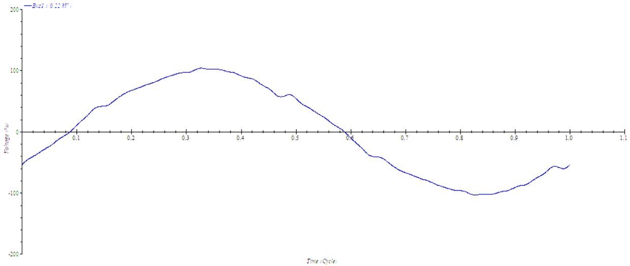
Figure 9. Sinusoidal Waveform Distortion on Bus 1
