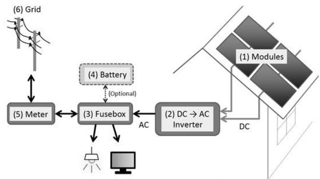
Figure 2. Direct current (DC) Power Plants are Connected to Alternating Voltage (AC) Electrical Networks via Power Electronic Devices [23]
