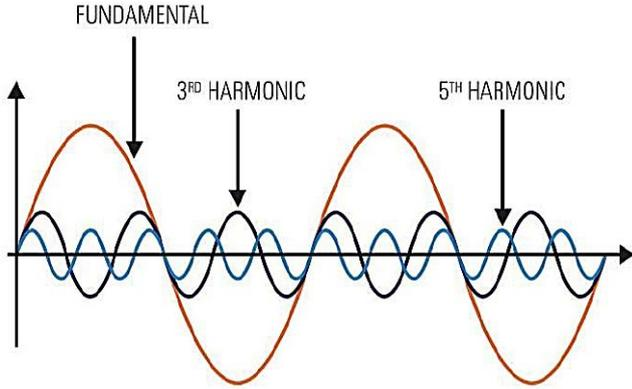
Figure 4. Fundamental Waves and Harmonic Waves
