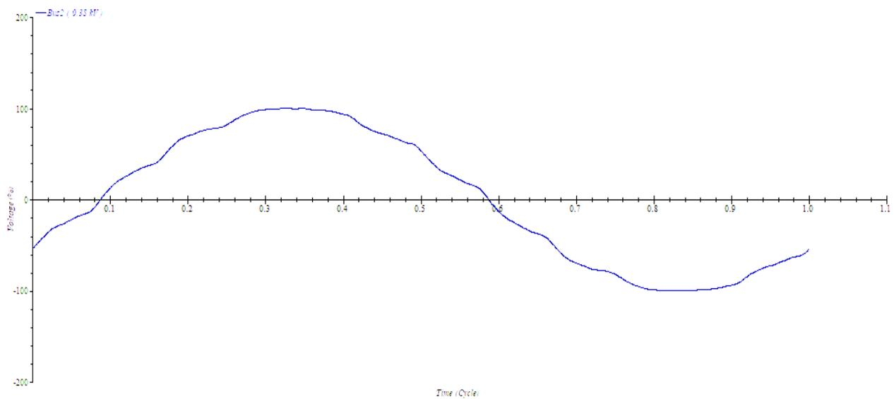
Figure 10. Sinusoidal Waveform Distortion on Bus 2
