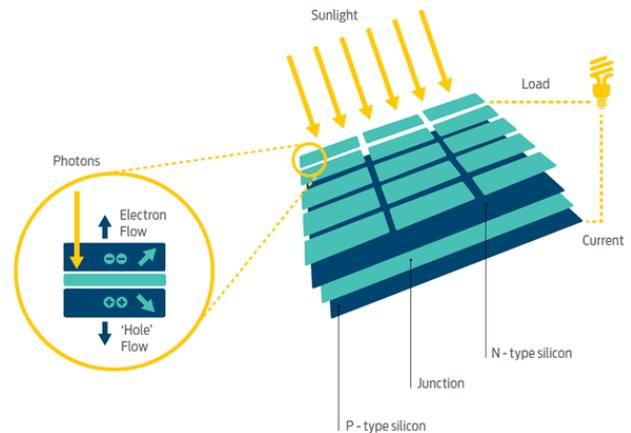
Figure 1. Working Principle of Solar Cells [22]
