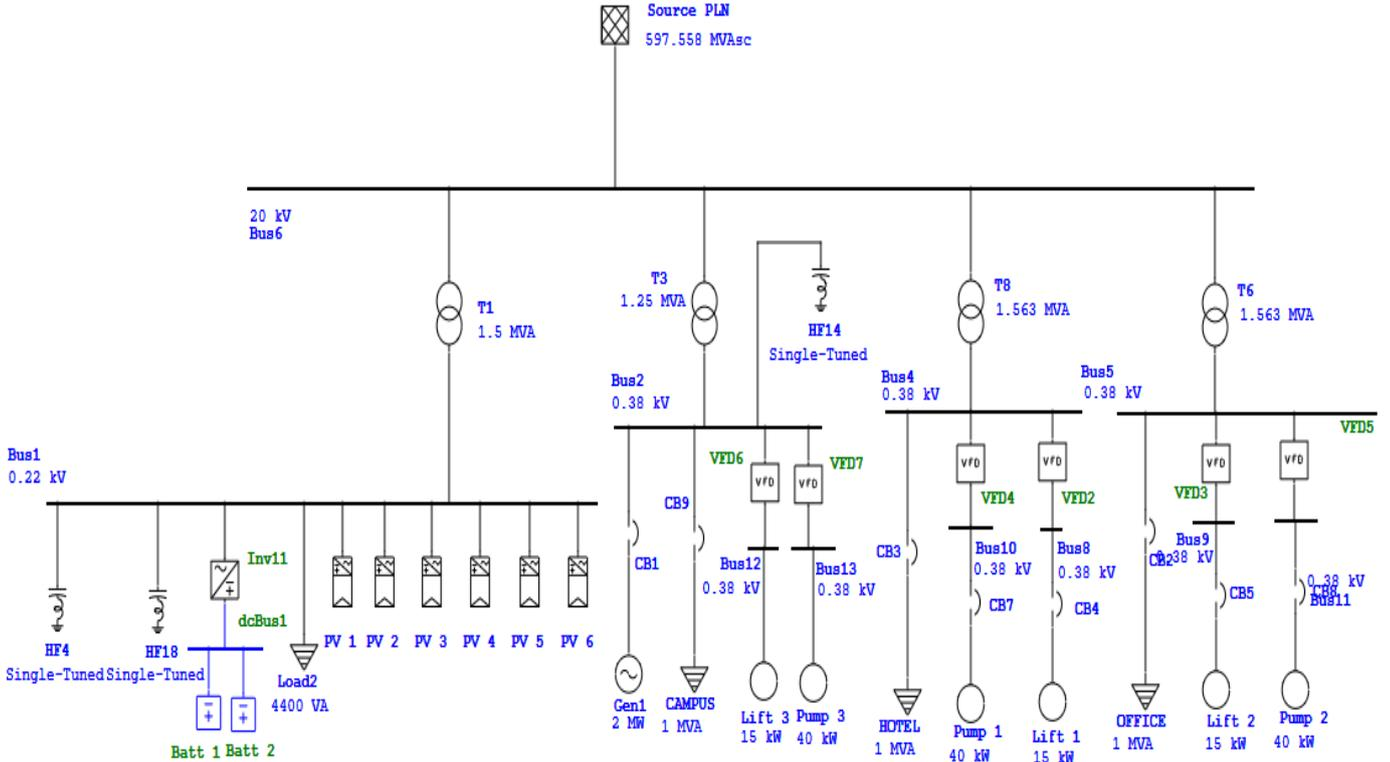
Figure 6. Single Line Diagram of Microgrid
