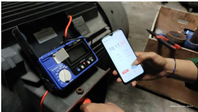
Figure 1. Insulation testing with a megohmmeter
