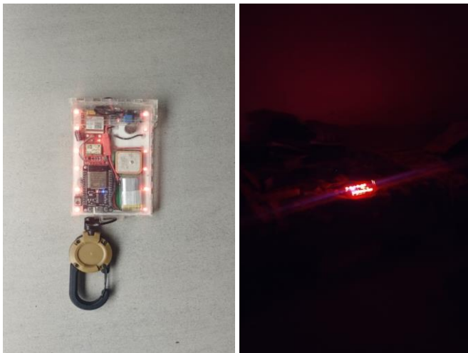
Gambar 9. Pengujian Visibilitas LED
