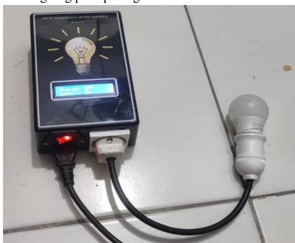
Gambar 4. Implementasi Sistem Kontrol Pencahayaan Berbasis Digital Addressable Lighting Interface (DALI)
