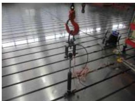
**Gambar. 5** Proses kalibrasi *shock absorber*
