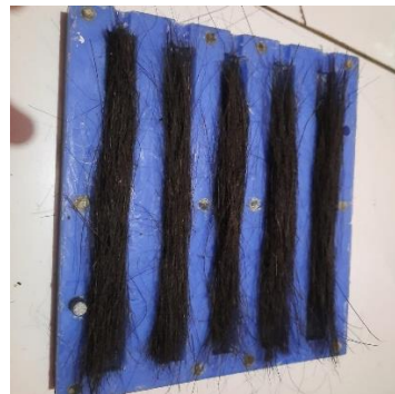
Figure 1. The Fibers Arranged Continuously in One Direction
