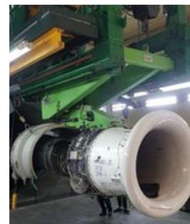
Gambar 2.4 Engine Adapter
