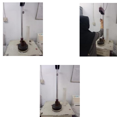
Figure 4. PE dart impact test uk 12 x 0.025
