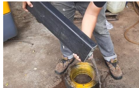
Figure 5 . Battery Electrolyte Drain
