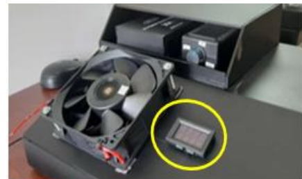
Figure 10. Battery Voltage Testing data capture
