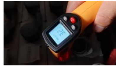
Figure 9. Retrieval of Battery Temperature Testing data
